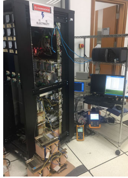
Fig. 9. Experimental setup of the 110 V–5 kVA SVC//HAPF experimental prototype.
